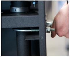
1. Level the box and securely fasten the U-bolt, do not over tighten.
