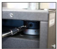
4. Ensure the silver shaft extension is inserted fully into the outer support shaft. Using the Long Allen Wrench that was included, securely tighten the set screw on the collar.
