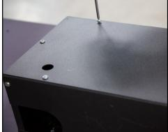
5. Reattach the cover that was removed in the beginning of Step:1 by reinserting all 6 screws. Align the hole on the cover with the set screw on the collar, in order to have access to adjust the height of the heating element.
