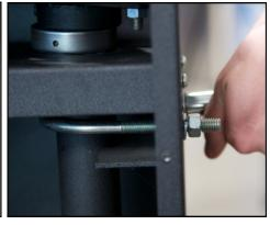
6. Slightly tilt the box forward so the black shaft fits into the half circle bracket. The silver collar sits on top of the bracket. Tighten the U-bolt evenly against the bracket.
