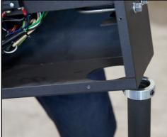
5. Check to confirm that the adjustment collar is set so the screw is facing forward and centered. Then place the box onto the outer shaft by inserting the shaft through the bottom opening.
