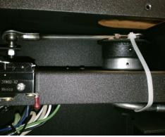
2. Inside the motor assembly, cut the plastic tie and remove the thrust bearing. DO NOT remove the collar that is attached to the actuator. Ensure the set screw on the collar is oriented outward.
