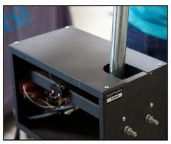
3. Insert the silver portion of the shaft into the top of the box. The shaft extension should pass through the collar, thrust bearing and into the outer support shaft (black shaft).
