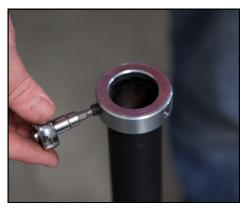
4. Add the replacement shaft collar to the top of the stand and tighten the two screws on the collar before installing the Auto Rotation Box.
