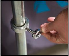
2. Make sure that the silver shaft has a collar tightened onto it. If not, slide the collar up the appropriate amount so that the collar can rest on top of the collar plate inside of the box, and tighten it.
